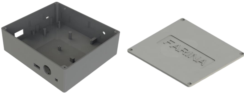
Figure 4.46. 3D modelling of case and cover designed with SolidWorks
