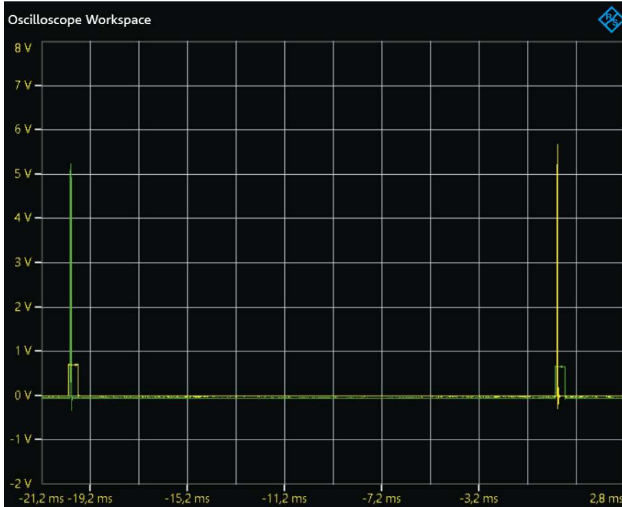
Figure 7.5: Macroscopic behavior: alternation of the transducers in the transmission and reception phases in the upstream and downstream cycles.
