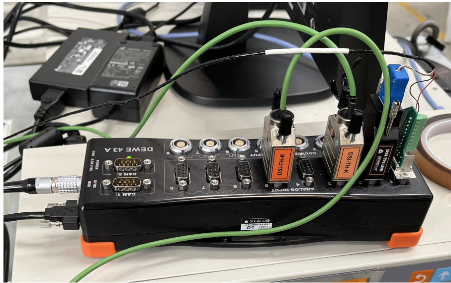
Figure 2.3: Detail of the data acquisition system wiring connections
