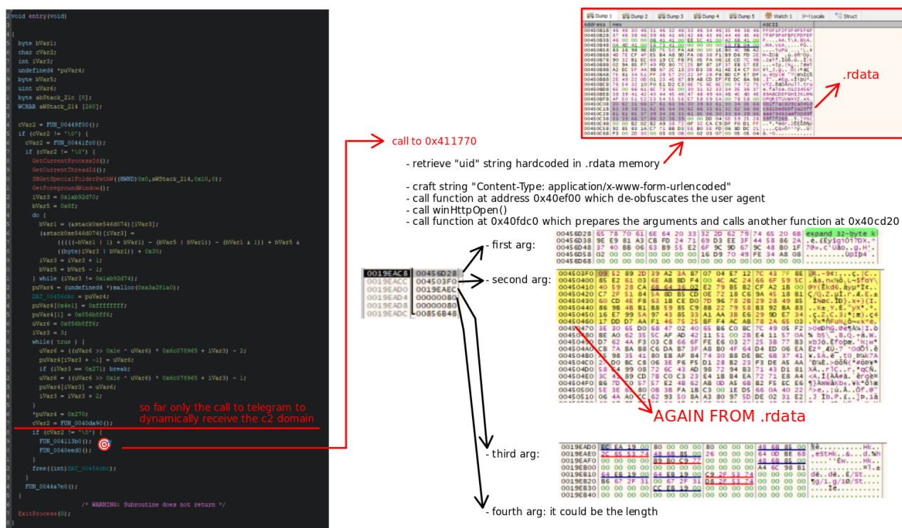
Figure 17: Visual representation of the execution flow leading to the invocation of the function at address 0x411770, as observed in x64dbg. The left side of the image displays the disassembled code path, while the right side highlights the contents of the .rdata section, including the hardcoded uid string and the suspected encrypted payload. The bottom section shows the four arguments passed to the decryption function, consisting of two pointers, an integer likely representing the input length, and an additional constant.
