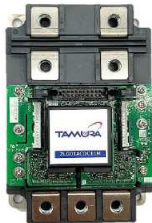
Figure 2.10: Example of an integrated gate driver unit directly mounted on an LV100 power module.
