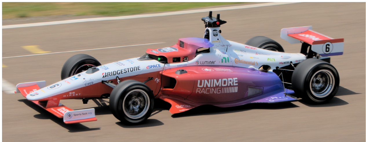
Figure 1.2: IAC Dallara AV24, an autonomous racecar based on the Dallara IL-15 Indy NXT chassis.
