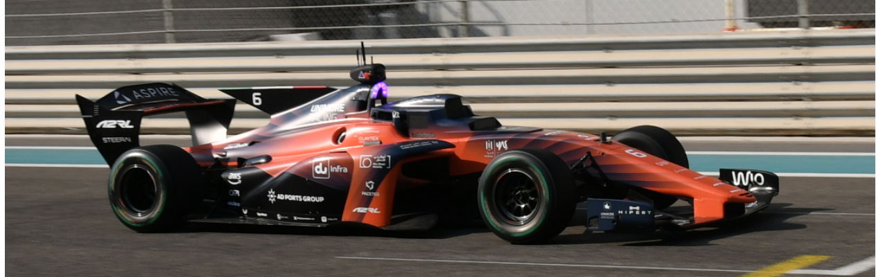
Figure 1.3: A2RL Dallara EAV25, an autonomous racecar based on the Dallara SF23 Super Formula chassis.
