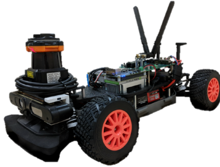
Figure 1.1: Roboracer, a low cost 1/10th scale autonomous racecar based on a modified Traxxas RC car.
