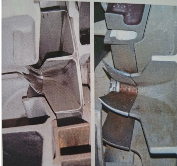
Figure 12: Hooker's reduced height impeller and Circular Arc Inducers
