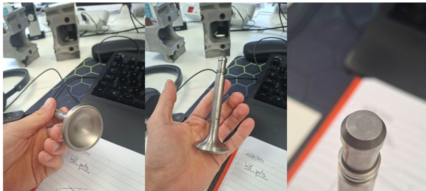
Figure 14: Merlin's sodium filled exhaust valves
