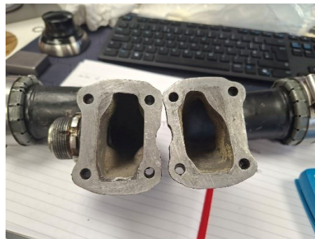
Figure 55: Elbows inlet section detail
