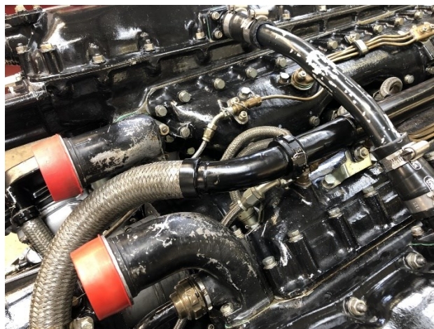
Figure 49: Hurricane's Merlin 500 with non-standard elbows (red cap)
