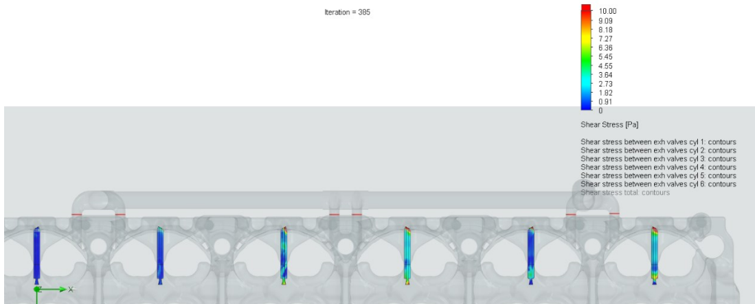
Figure 79: Shear Stresses between exhaust valve seats bottom view
