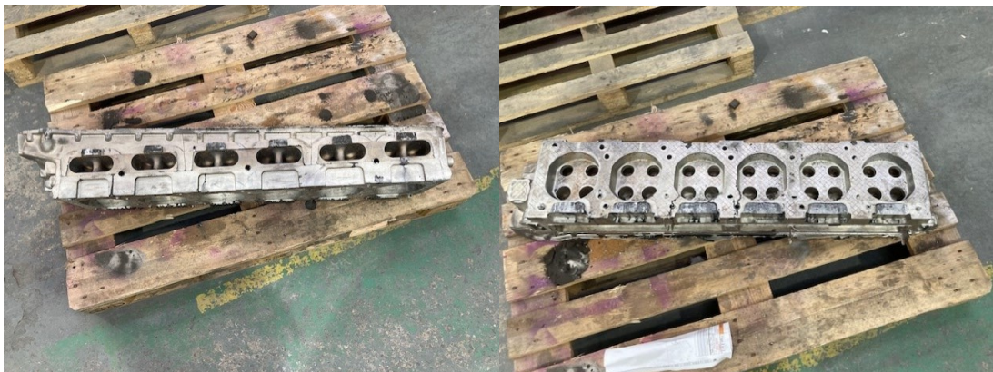
Figure 43: Brand new A bank out of the sand mould
