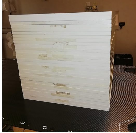
(b) 30 cm water-equivalent slab phantom setup.
