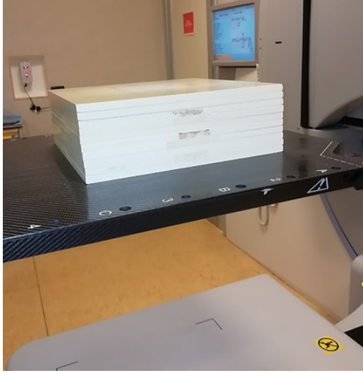
(a) 10 cm water-equivalent slab phantom setup.
