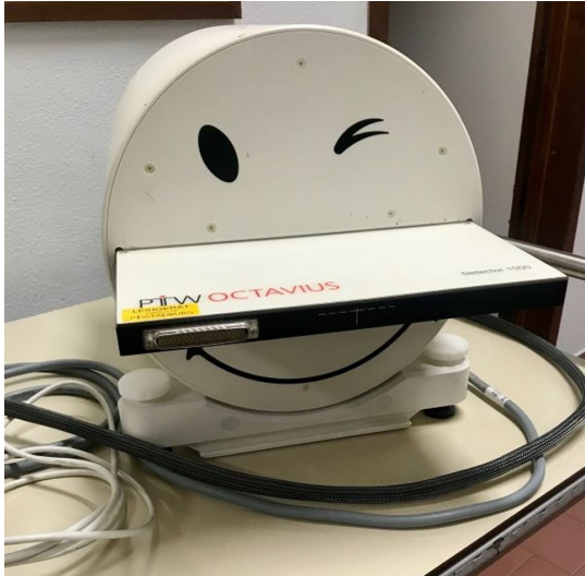
(a) OCTAVIUS cylindrical phantom used for patient-specific QA measurements.
