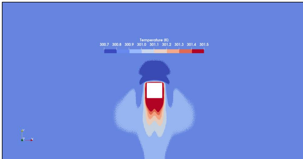
FIGURE 4.16 Case C — active: buoyancy lifts heat upward, reducing temperature at pedestrian level in the wake. The thermal field is more confined to the immediate vicinity of the heated surfaces. Range 300.7–301.5 K.
