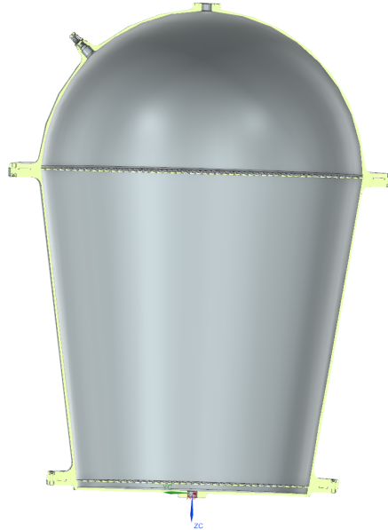
Figure 6.20: Reactor tower section
